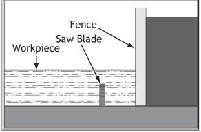
Figure 28. Example of a non-through cut.
